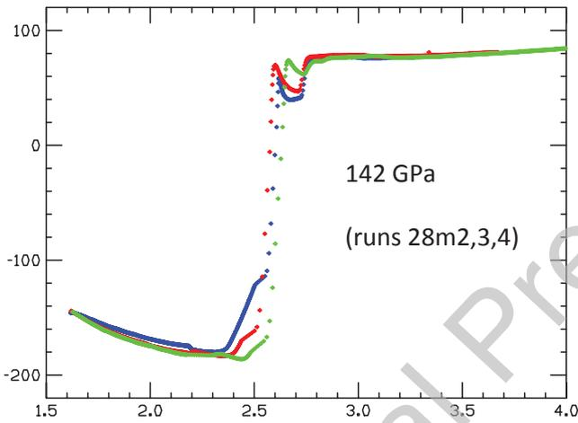
FIG. 8: All the warming runs obtained from the raw data for pressure 142 GPa. The horizontal axis shows temperature in K and the vertical axis shows real part of the ac susceptibility in nV. The vertical shift relative to the data shown in Fig. 7 has no physical significance.
