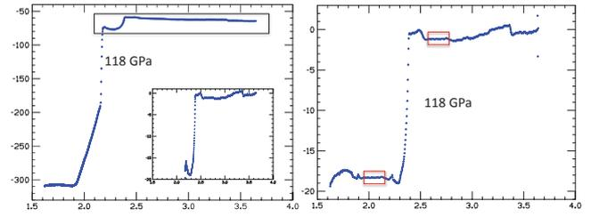
FIG. 9: The right panel shows the published curve for 118 GPa. The left panel shows the measurements for 118 GPa (file 102008m2.dat) after background subtraction. The inset of the left panel shows the part of the curve enclosed in the rectangle after subject to the transformation  $ch_{inew} = chi + 46.842 + 4.836T$ . Note that the inset on the left panel looks identical to the upper part of the curve on the right panel.
