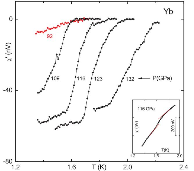
FIG. 2: Ac magnetic susceptibility of Yb under pressure ([7]). The inset shows raw data, from which the signal shown is extracted by subtraction of a background signal.
