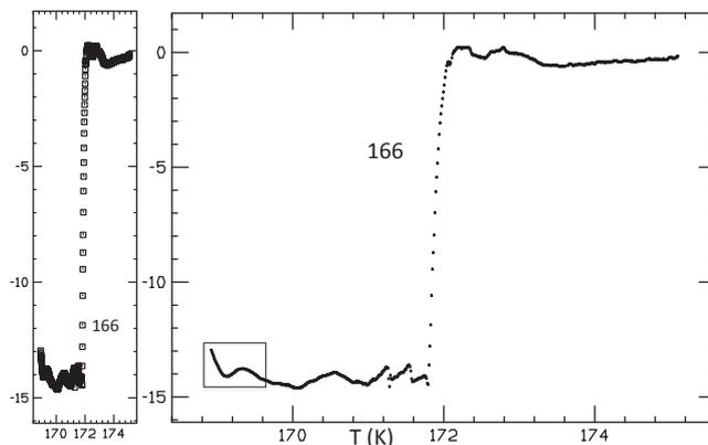
FIG. 12: Susceptibility data for CSH at 166 GPa plotted with the resolution of ref. [1] and with higher resolution.
