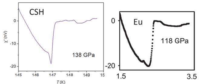
FIG. 4: Raw data for ac magnetic susceptibility of *CSH* [1] and of *Eu* [10] under pressure.
