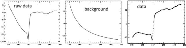
FIG. 5: Attempt at modeling the reported raw data for CSH. The left panel shows the reported raw data [1]. The middle panel shows an assumed background signal corresponding to Curie-Weiss behavior with Curie temperature 143.9K, i.e. only 2% away from the assumed superconducting  $T_c = 147K$ . The right panel shows the resulting data obtained from subtracting the background signal from the raw data, Eq. (1).
