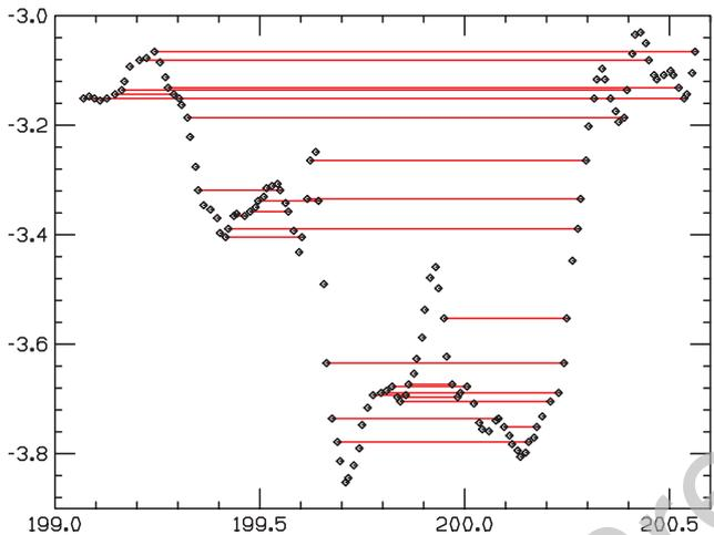
FIG. 15: Part of the susceptibility data for CSH at pressure 189 GPa (enclosed in the rectangle in Fig. 14), showing many points for which the susceptibility is the same to 6 digits accuracy, connected by red lines. There is one case of seven points on the same red line, for which the susceptibility is the same to 6 digits accuracy, shown in more detail in Fig. 16.
