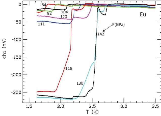
FIG. 7: Real part of ac susceptibility versus temperature for Eu metal as pressure is increased from 84 to 142 GPa. One warming run for each pressure was selected from the raw data, then the background signal was subtracted.
