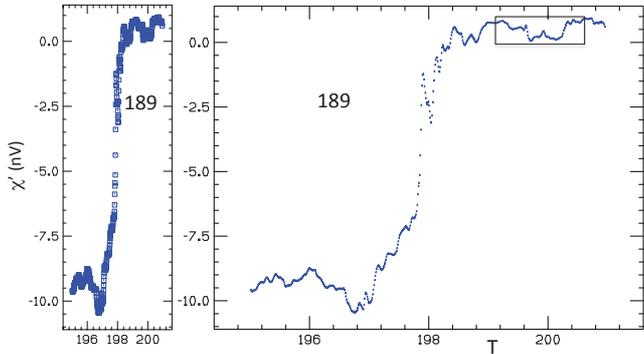
FIG. 14: Susceptibility data for CSH at 189 GPa plotted with the resolution of ref. [1] and with higher resolution.
